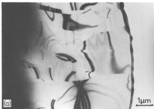
Figure 1 (a) A typical thin crystalline region in as-splatted Al-17.3 at.% Cu; (b) selected-area diffraction pattern from a single grain.
